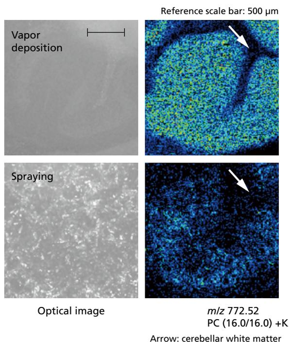
Achieves improved resolution and a matrix coating uniformity impossible using the spray method.
