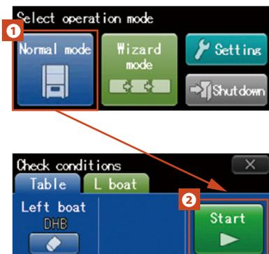
After system startup, press (1) and then (2) to start deposition.
