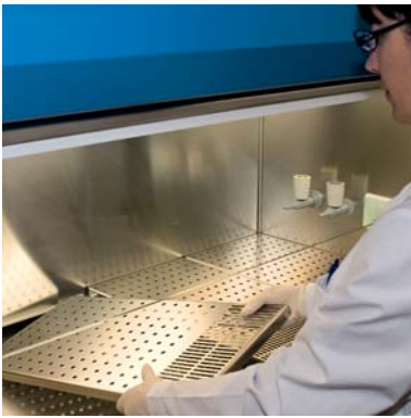
REMOVABLE WORK SURFACE Work Surface in stainless steel AISI-316L, consisting of sections which are easily removable for carrying out routine cleaning and/or require autoclaving sterilization procedures; perforated to ensure an optimum degree of laminarity of the airflow, together with a high resistance factor to the most effective chemical agents used for disinfection. Single piece work chamber Work chamber in stainless steel AISI 304L, designed to fulfill the requirements and pass the "cleanability tests" according to EN12469:2000.
